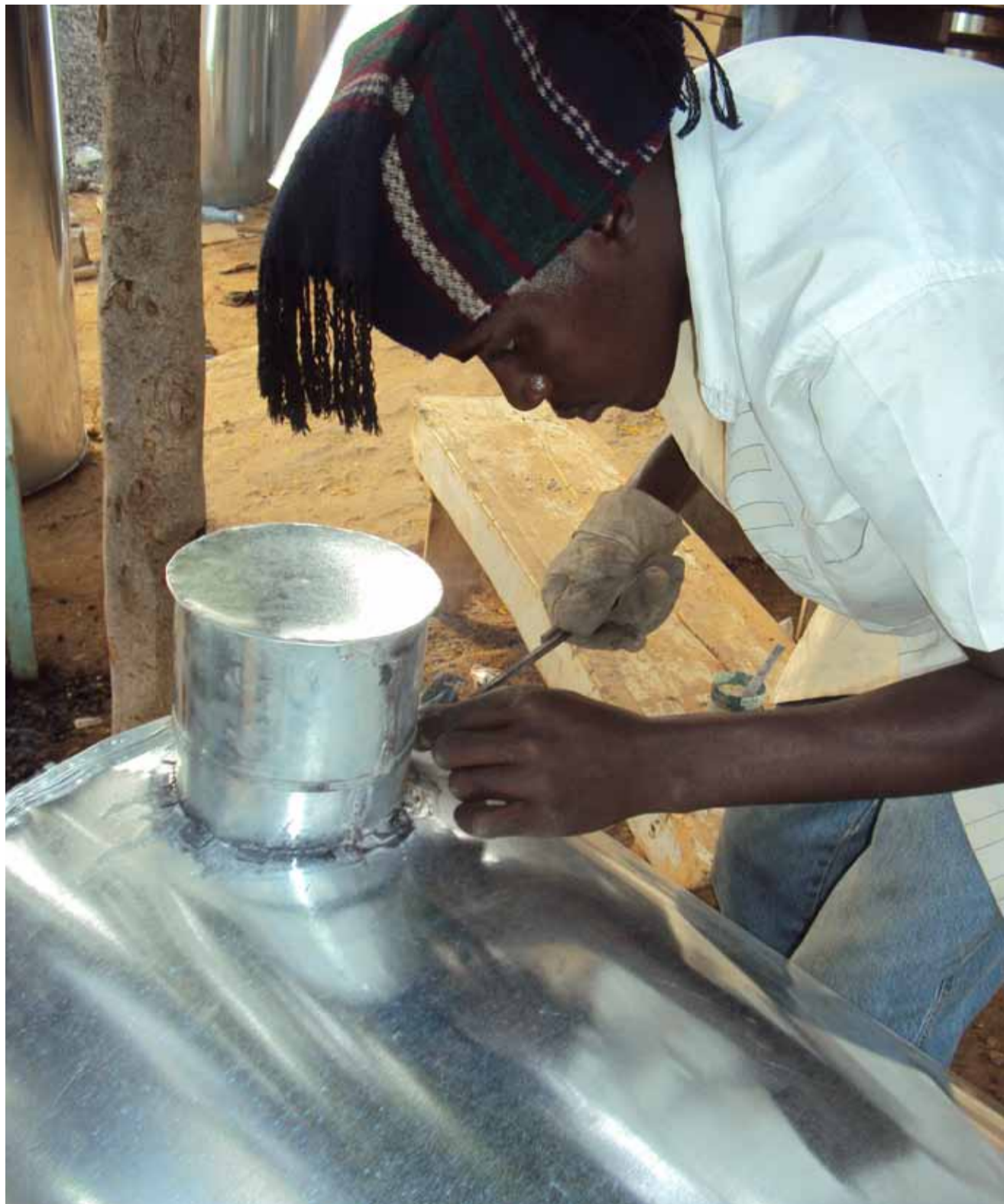
A skilled artisan puts the finishing touches on a metal grain silo. ©FAO/Dan Irura
